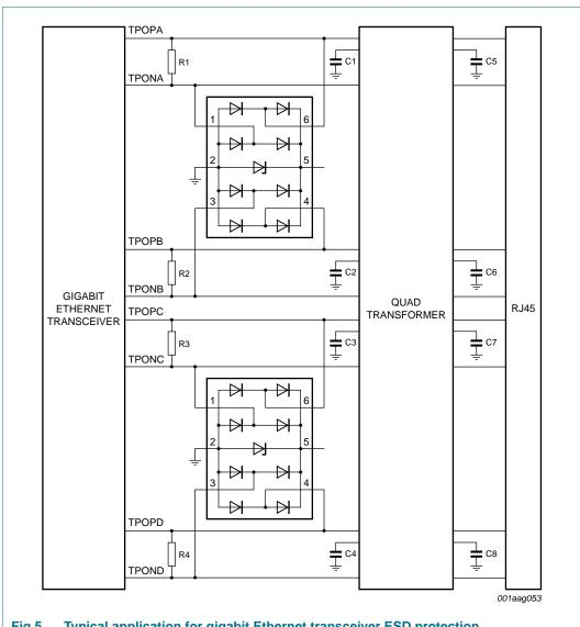
Typical application for gigabit Ethernet transceiver ESD protection Fig 5.
