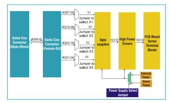
For more information on Stackable Stepper Motor Controller Snap On board, visit http://slscorp.com/pages/steppermotorsls.php
