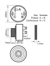
The AE20M Piezo Buzzer Series offers an economical and cost effective solution for local area applications. At only 43mm diameter, the buzzer offers the installer an unobtrusive accoustic signal in a wide range of voltages with most voltages offering pulsed or continuous tone capability.
