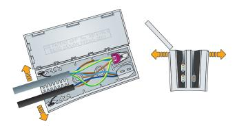
Try to keep cables of a similar size together in the same slot and simply push them into the slot as far as they will go.
