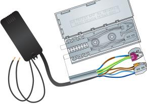
When fitting the cables into the cable clamp the sides of the box need to be eased apart to make an opening. It is normal for the entrance to be splayed apart with the cables in place.
