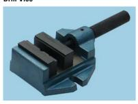
Small drill vice for use in drilling and light milling operations. Effectively grips round, square, thin and irregular sections. The jaws are made of hardened steel and base cast iron. Handle is mounted on ball bearings to give more gripping power, smooth action and long life.
