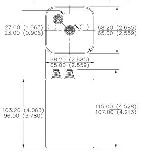
THIS BATTERY SHALL PASS FREELY THROUGH A CYLINDRICAL TUBE 82.6 DIAMETER X 101.6 LONG.
