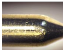
Han ® D contacts with GoldTec surface after 500 mating cycles.
