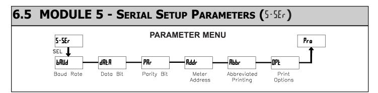
The Serial Setup Parameters are only active when the optional RS232 or RS485 serial communications module is installed in the meter. Refer to the CUB5COM bulletin for complete details on CUB5 serial communications.
