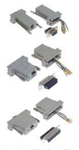
Adapts male or female DB9, DB15 or DB25 computer plugs to 8 position RJ45 or 6 position RJ11 modular socket. Back shell is pre-wired to modular socket ready to insert pins into desired positions of the DB connector.
