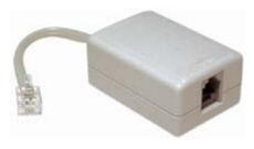
An ADSL filter is required on an ADSL line between each analog device (telephone, fax machine, fax/modem, modem, cordless telephone, alarm dialer etc) and the associated wall outlet. If a filter is not installed, your voice-calls will experience interference whenever ADSL data is being transmitted. Our K2310ASH ADSL Line Filter is ADSL2 and ADSL2+ compatible.
