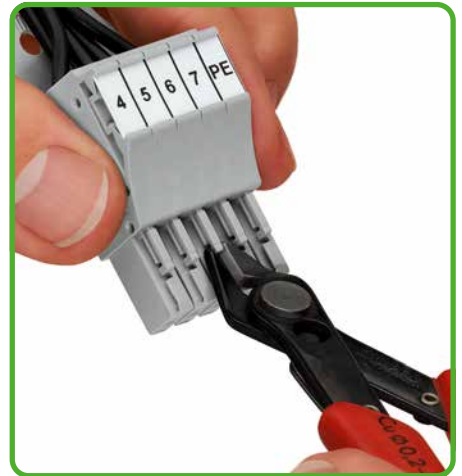
To code a female plug, remove the desired coding finger using a suitable tool.
