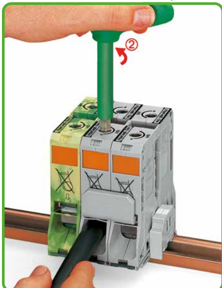
Unlock the locking tab with a short counter-clockwise turn ② of the Allen wrench to securely terminate the conductor.
