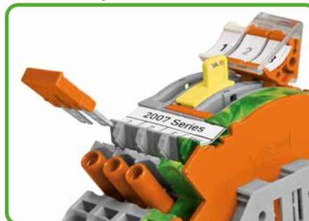
Additional commoning option via circuit-related jumpers or testing via test plug adapters (209-170) on transformer side
