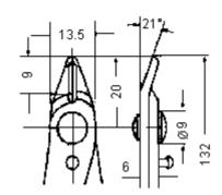
Cutting Capacity: 14 AWG (11.6 mm)
