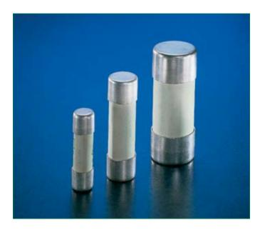
Littelfuse fast acting (gL-gG) fuses are used for the protection of cables against short-circuits. Time-lag (aM) fuses are used for protection of motors.
