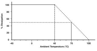
Dissipation as a function of temperature. Potentiometers covered by this specification are derated from 100% rated dissipation at 40°C to zero dissipation at 100°C.
