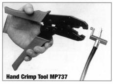
The hand crimp tool has interchangeable die sets for various sizes of cable, see table for correct die set code.
