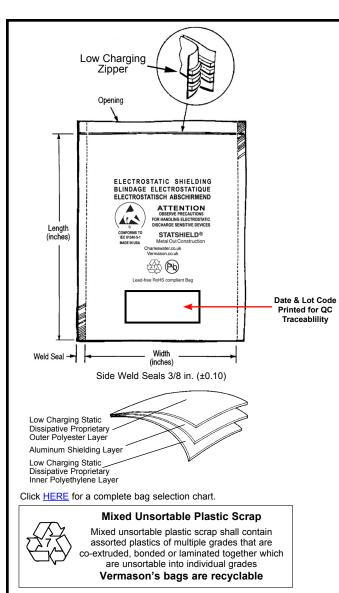
Statshield<sup>®</sup> bags are packaged 100 per package in an oversized shielding bag. Shelf life of bags is minimum one year in normal indoor storage conditions. See <u>Statshield Bag Storage Information</u>.
