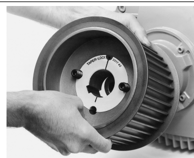
INSERT SCREWS and LOCATE ON SHAFT
