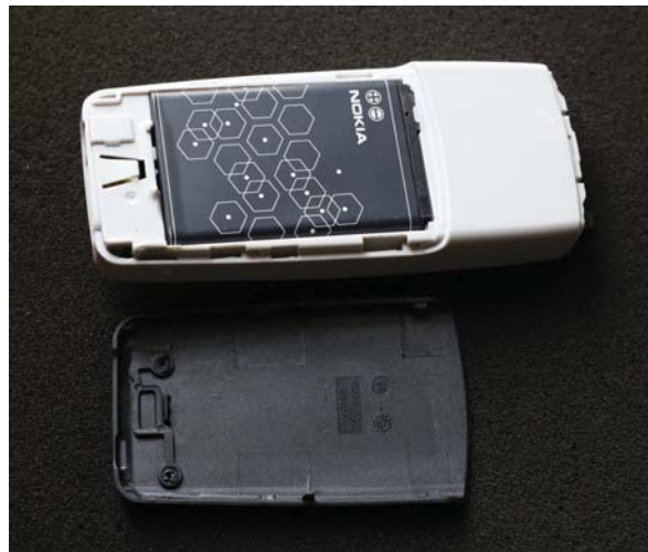
Figure 7. Nokia BL-5C Li-ion Battery Mounted Inside Back-cover of the Main Unit
