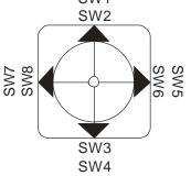
Two switches will actuate in each of the four directions: North, South, East & West.
