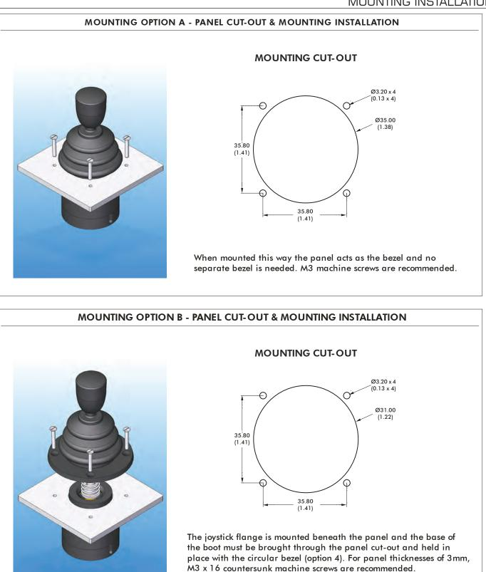
Note: When sub panel mounting, great care should be taken not to damage the boot, or any of the mechanism under the boot. All panel cut-outs should be free from sharp edges and swarf that may damage the boot.
