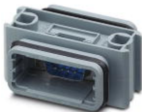
D-SUB coupling, shell size 1, pin, gender changer, shielded, connection direction straight, IP67 degree of protection
