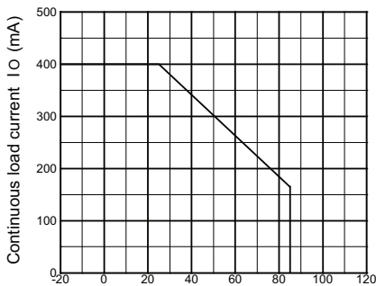
Continuous load current vs. Ambient temperature I_O - T_a
