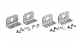
Used to provide best load distribution while lifting two or three ganged enclosures with up to 1000 lb. of equipment and cabling in each bay. Angles mount to top of enclosure frame corner blocks and do not require removal of top cover for installation. Kit consists of two angles and four bolts and washers. Angles are clear zinc-coated 10 gauge steel.
