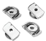
Twenty plated clamping nuts with top-grip nut retainers. Clamping nuts fit into mounting channels that are used on inside walls of Hoffman enclosures. Clamping nuts are included with all Hoffman accessories that attach to mounting channels. These clamping nuts can be used for mounting other equipment (brackets, etc.) to the enclosure walls.
