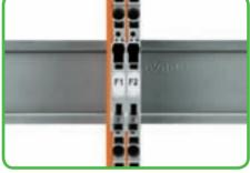
Fuse terminal blocks with a width of 6.2 mm/0.244 in can be assembled adjacent to each other. At the end of an assembly, if there is **no** adjacent fuse or disconnect terminal block, an end plate for fuse erminal blocks must be used.
