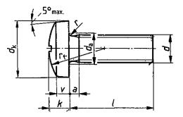
Raised cheese head screw, with unthreaded portion of shank\* (below the stepped line in the table)
