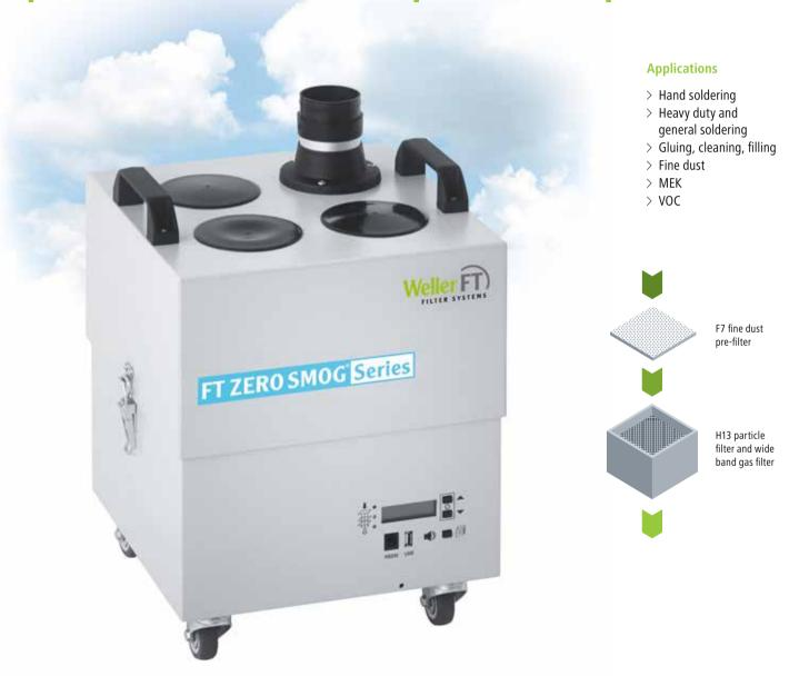
The fume extraction unit Zero Smog®4V (ZS4V) is easy to install and operate. The kit is supplied with one flexible hose, one attachment arm with funnel and one bench mount bracket ready for installation at the workplace. A powerful, maintenance-free turbine provides continuous fume extraction at a maximum air extraction rate of 230 m3/h. When setting the Constant Flow Control, the adjustable turbine speed avoids unnecessary waste of power and saves energy.
