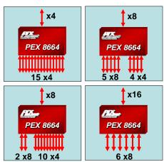
Figure 1. Common Port Configurations
