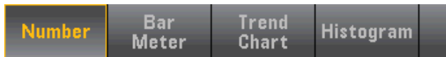
Figure 1. When you press the Display button, the soft keys show the choices available for the different display modes.
