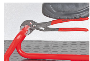
Teeth set against the direction of rotation have a self-locking effect and prevent slipping on the workpiece.
