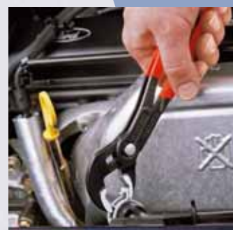
Gripping surfaces with special hardened teeth for secure gripping of differently shaped workpieces
