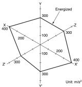
Sample: G6B-1114P-US Number of Relays: 12 pcs Test Conditions: Shock is applied in  $\pm X$ ,  $\pm Y$ , and ±Z directions three times each with without energizing the Relays Shock direction to check the number of malfunctions. z 💿 Requirement: None malfuction 100 m/s<sup>2</sup> (Coil)
