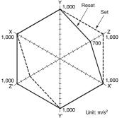
Sample: G6BK-1114P-US Number of Relays: 12 pcs Test Conditions: The value at which malfunction occurred was measured after Shock direction applying shock to the test piece 3 times each in 6 directions along 3 z 💿 axes. Standard value: (Coil) 300 m/s<sup>2</sup>
