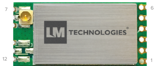
RF Type 1: IPEX Connector Module
