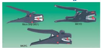
A range of automatic wire strippers to cover cable sizes  $0.25 mm^2$  to  $6.00 mm^2$ . They all operate using a unique system of self adjusting multiple blades which slice cleanly through the insulation but then form around the conductors to give a clean cut without causing any damage.
