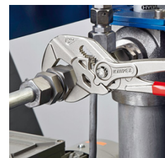
replaces the need for sets of metric and imperial spanners
