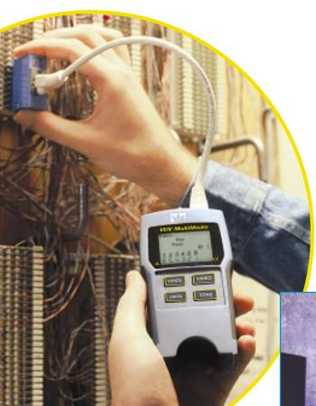
Users can quickly move through Voice, Data, Video/Security networks, testing all wiring types using the same tester.
