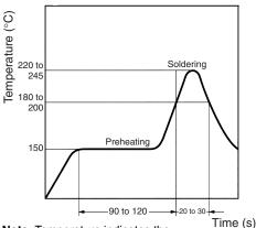
**Note:** Temperature indicates the surface temperature of the PCBs
