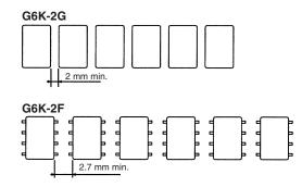
Two or more Relays may be mounted as closely as desired with the short sides of the Relays facing each other.
