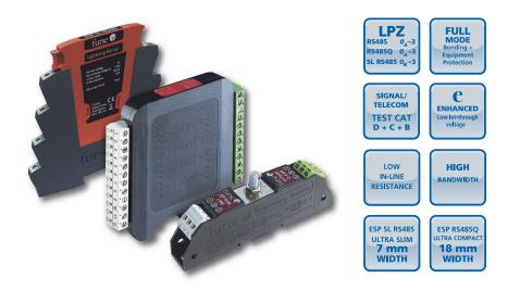
Combined Category D, C, B tested protector (to BS EN 61643) specifically designed for RS 485 and Fieldbus applications, such as Profibus DP. For use at boundaries up to LPZ  $0_A$  (ESP RS485 & ESP RS485Q), or LPZ  $0_B$  (ESP SL RS485) protect against flashover (typically the service entrance location) through to LPZ 3. Available as standard ESP RS485 format, or compact ESP RS485Q and Slim Line ESP SL RS485 versions for installations where a high number of lines require protection.
