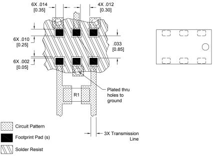
Dimensions are in Inches [Millimeters] Mounting Footprint
