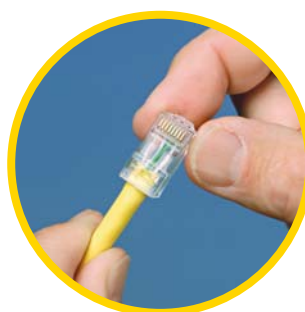
STEP 7 Slide assembly into plug body.
