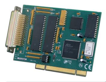
The PCI-PIO is a PCI-compatible half-card which provides digital input/outputs and counter/timers. There are 48 TTL-compatible programmable digital input/outputs available from the board. If the controlling devices are used in handshake mode, the handshake lines are available as interrupt sources.
