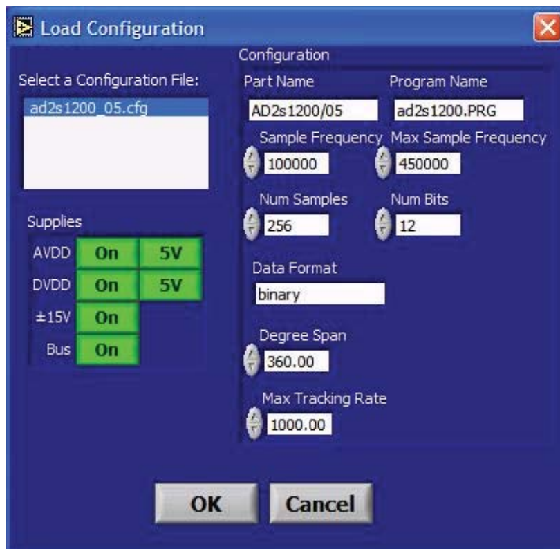
Figure 4. AD2S1200/05 Evaluation Software, Load Configuration Window
