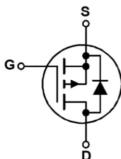
Please Note: These lateral mosfets do not include a G-S protection network and care must therefore be taken with static handling precautions and the appropriate protection in the amplifier circuit. Please refer to the application notes for more information.
