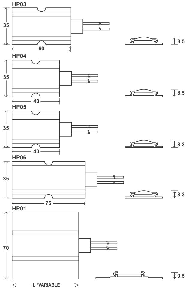
The DBK HP range of Positive Temperature Coefficient (PTC) self regulating heaters have been designed to offer a wide choice of power outputs within a compact series of aluminium profiles. These elements can be operated without the aid of a thermostat or thermal cut-out.
