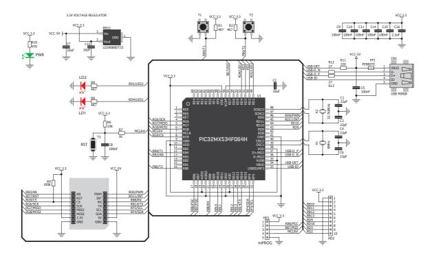
Figure 1-2: PIC32MX clicker schematic
