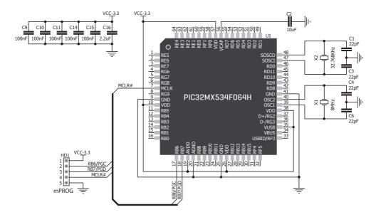
Figure 4-10: mikroProg<sup>™</sup> connection schematic
