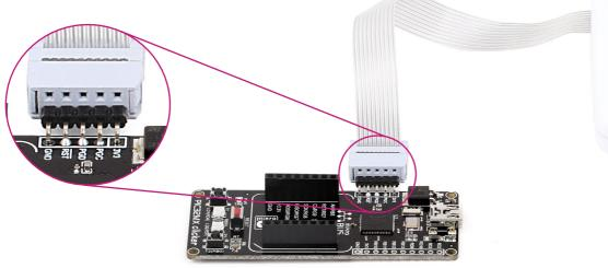
Figure 4-9: mikroProg<sup>™</sup> connector
