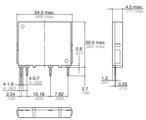
General tolerance:  $\pm 0.2 \pm .008$ **PC board pattern (Bottom view)**
