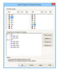
The 16 digital inputs can be added to the view by dragging and dropping, and can then be reordered, grouped, and renamed. The channels can be displayed individually or in arbitrary groups labelled with binary, decimal or hexadecimal values. A separate logic threshold from -5 V to +5 V can be defined for each 8-bit input port. The digital trigger can be activated by any bit pattern combined with an optional transition on any input.
