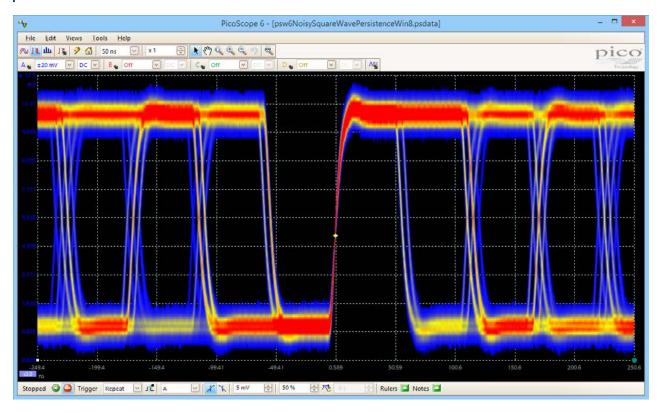
Color Persistence mode allows you to see old and new data superimposed, with new or more frequent data in a brighter color or shade. This makes it easy to see glitches and dropouts and to estimate their relative frequency. Simply click the persistence button and choose between analog intensity, digital color, and fast display modes, or create your own custom rules.
