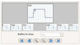
When the trace length is set to be shorter than the scope's memory, the PicoScope will automatically configure the memory as a circular buffer, recording recent waveforms for review. For example, if 1 million samples are captured, up to 500 waveforms will be stored in oscilloscope memory. Tools such as mask limit testing can then be used to scan through each waveform to identify anomalies.
