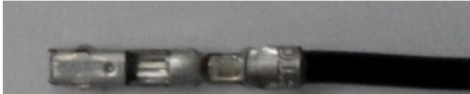
Fig.1: Showing female contact back side
