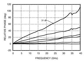
Step Attenuation vs. Attenuation State 18 - 30 GHz
