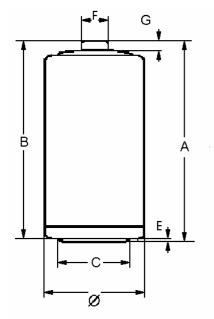
Type Designation 4920 **Designation IEC LR20** Zn-MnO<sub>2</sub> (Alkaline) System Shelf Life (Coding)\* 5 years Nominal Voltage [V] 1.5 Typical Capacity C [mAh]  $16500 \; (\text{discharge with high-resistance})$ Permissible Temperature Range - 10 °C ... 50 °C Weight, approx. [g] 144 Volume [ccm] 51.3 Dimensions [mm] min: max: Ø 34.2 32.3 A B C E 61.5 59.5 18.0
