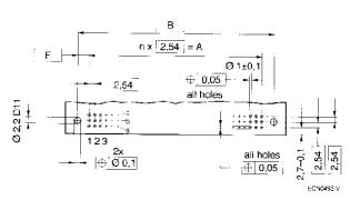
Mounting Holes (component side) for Printed Circuits. (For connectors with soldering pins angled at 90°.)
