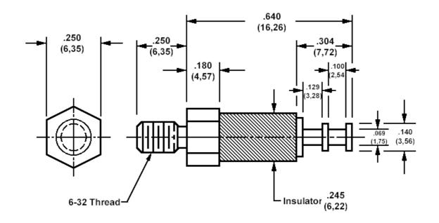
How to order code  $\underline{570\text{-}1504\text{-}01}$ - $\underline{YY}$ - $\underline{19}$  Basic Part No (YY = plating finish. See tables for options)
